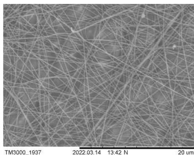
Fig. 3. Morphology of nanofibers collected in stationary plate
