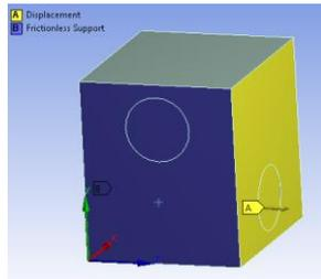
Fig. 9. **Boundary conditions in biaxial longitudinal model**
