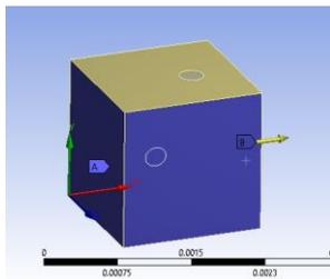
Fig. 11. **Boundary conditions in random fibre longitudinal model**
