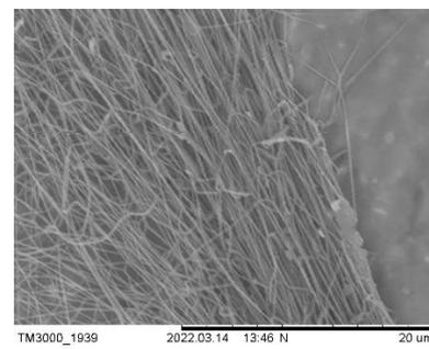
Fig. 4. Morphology of nanofibers collected in rotating drum
