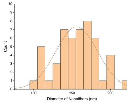
Fig. 6. Diameter of nanofibers collected from rotating drum
