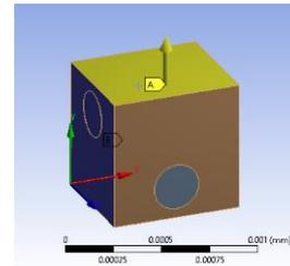
Fig. 10. **Boundary conditions in biaxial transverse model**
