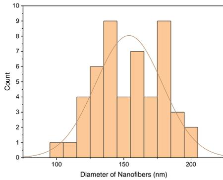
Fig. 5. Diameter of nanofibers collected from stationary plate
